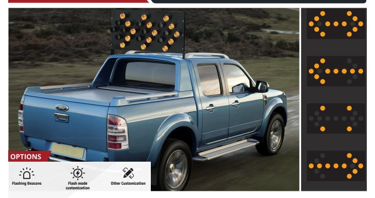
The Vehicle Mounted Arrow Board allows for mounting over any vehicles with actuators and brackets, foldable and easily operated. It is built to meet CE & AS Standards, with wide angularity and superior visibility, provide an obvious solution for convoys, crashcushion (TMA) trucks and emergency repair crews.
